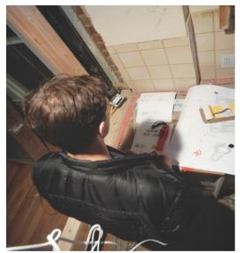
Enlisting the help of his client Mike, and use of Mike's under-construction kitchen, the author (on ladder, left) measured foot-candles delivered from 4- and 5-inch recessed cans and several different bulbs. With Mike standing at the counter, light levels from fixtures located beyond the counter edge dropped dramatically because of shadows cast on the work surface (right).
