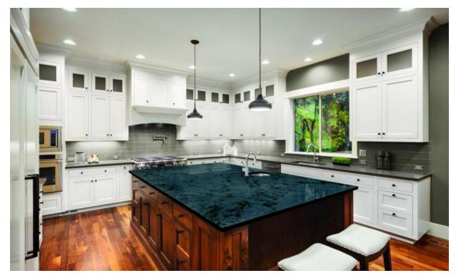
What's wrong with this kitchen lighting scheme? Can lights located in aisles cast shadow on tasks when the cook stands at the counter. Under-cabinet lights mounted against the wall cause glare. There are too few fixtures to light an island of this size. Read on for solutions that will bring better lighting to your kitchen designs.
